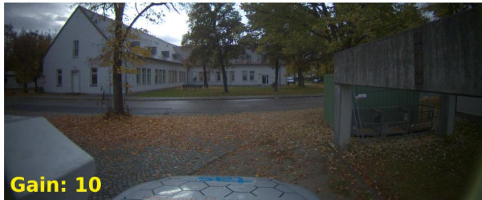
The same scene for different Gain and a fixed exposure time of  $2000\mu\text{s}$ .
