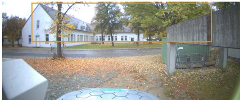
The same scene with different areas of the image used for the internal auto exposure control.
