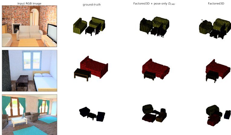
Figure 8 Comparison of the object prediction of the original Factored3D network to the extension using the point cloud based D_{EMD} as loss function on the rotated shape prediction.
